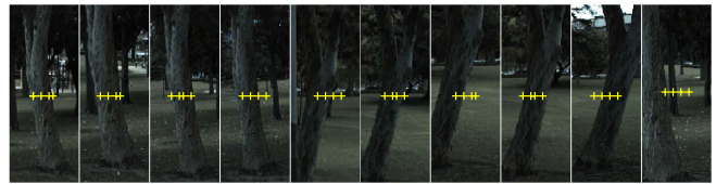
Fig. 5. Multiple views of one of the landmarks acquired during SLAM. As with this particular landmark, during outdoor exploration, the vehicle observes landmarks at completely different viewpoints. The yellow crosses represent laser points projected on the object. As laser scans and images are not perfectly synchronised, misalignment exists especially when the vehicle is turning (last image on the right).
