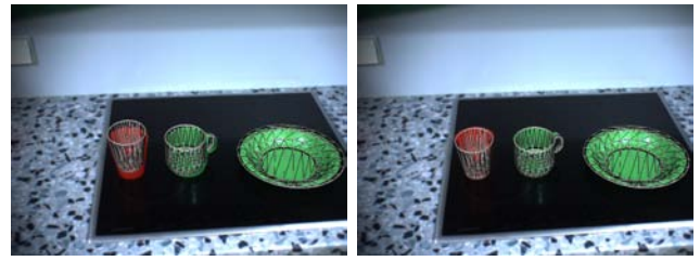
Fig. 4. Effect of the position correction on an example scene. Left: with orientation correction only. Right: with orientation and position correction.
