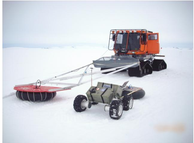
Fig. 1. The Yeti robot next to the Tucker Sno-Cat. Yeti will supplement or replace the Sno-Cat for performing Ground Penetrating Radar Surveys to detect sub-surface crevasses in polar ice sheets.
