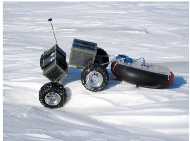
Fig. 2. A passive pivot linking the front and back half of the Yeti robot chassis allow it to maintain four-point contact on rough terrain.
