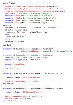
Figure 5: Modelica program code for the model of tank2.
