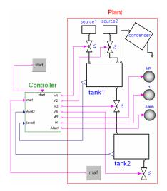
Figure 1: Scheme of the evaporator system.
