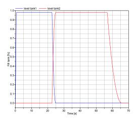
Figure 6: Level tanks in function of time in normal operation of the evaporator system.
