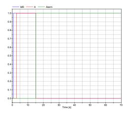
Figure 9: Switch state of the mixer, heater and alarm with occurrence of condenser malfunction (time =15s).
