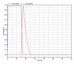
Figure 8: Level tanks in function of time with occurrence of condenser malfunction (time = 15s).
