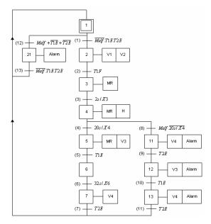
Figure 2: SFC of the system controller.
