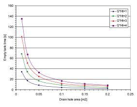
Figure 10: Empty tank time in function of plant variables.
