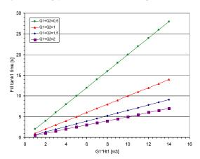
Figure 11: Fill tank1 time in function of plant variables.
