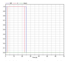
Figure 7: Switch state of the mixer, heater and alarm in normal operation of the evaporator system.
