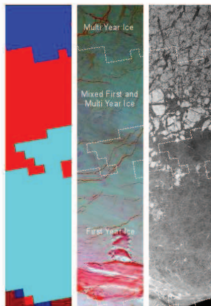
Figure 1: Comparison of images from 31 March 2007. From left to right: Cluster analysis of data from all 7-channels of SSM/I (NSIDC daily gridded brightness temperature data); MODIS false colour composite (infrared channels) from 21:20 UTC (NASA); and, Envisat ASAR WSM from 06:37 UTC (ESA)
