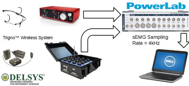
Figure 1. The system setup for data collection
