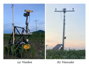
Figure 1: The developed platforms for high-throughput phenotyping in the field deployed at the Bradford Research Facility: (a) ground vehicle, Vinobot; and (b) observation tower, Vinoculer shown at the height of 15ft
