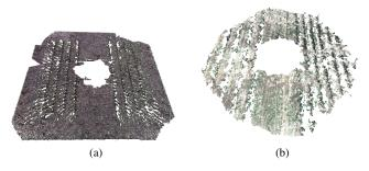
Figure 6: Results for the 3D reconstruction of the entire field by Vinoculer using (a) simulated and (b) real data
