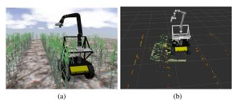
Figure 3: (a) Simulation of Vinobot in the field using Gazebo, and (b) Visualization of the real Vinobot and sensor data by Rviz. The orange points are parts of the plants detected by the LiDAR. The figure also displays the 3D point could being created by the stereo camera handled by the robotic arm.
