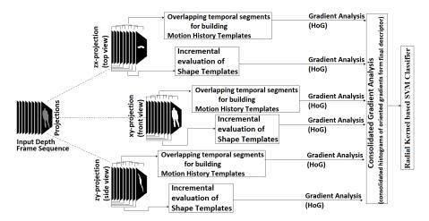
Fig. 1: Process flow for the proposed 3D activity recognition approach.
