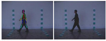
(a) the human pose estimation result by (b) because Ferrari's upper-body detecour method tion method cannot detect the upper body, nothing is attained
