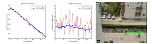
**Fig. 5.** The output path of detector and tracker. The first two plots are the path of x direction and y direction, the third figure is trajectory diagram of the video 'Walk'.
