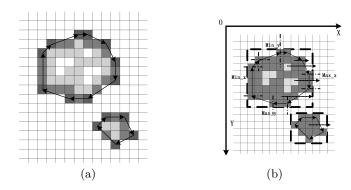
Fig. 3. In (a), the mesh blocks, grey blocks and twill blocks are the Mask after filtering in motion vector field, the grey blocks represent the boundary blocks on the boundary searching, the intermediate-blank blocks represent the missing blocks, and the mesh blocks are convex hull points. In (b), the rough borders are searching area, whose internal is used to fill points by ray method for avoiding repeated searching.
