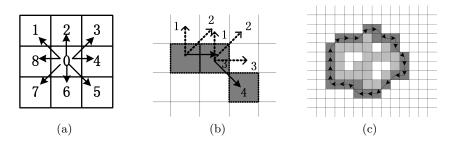
**Fig. 2.** Adaptive boundary blocks scanning. (a) Eight-direction template. (b) the scanning order of the eight-direction. The dotted lines and serial numbers represent the order of scanning. (c) The grey blocks represent the boundary blocks after scanning.
