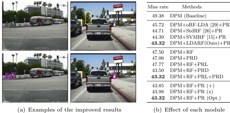
Fig. 7. Effects of the expert model. (a) Sampled results of Straightened detection at 1 FPPI ([ Top ] DPM [7], [ Bottom ] Ours (DPM+LDARF+PR)). We denote the false positives and true positives as Yellow and Magenta respectively. (b) Comparisons according to the expert types ( Top , Sec. 3.2), the perspective-aware rejection scheme in the learning and detection step ( Middle , Sec. 4), and integration rules ( Bottom , Sec. 3.3)
