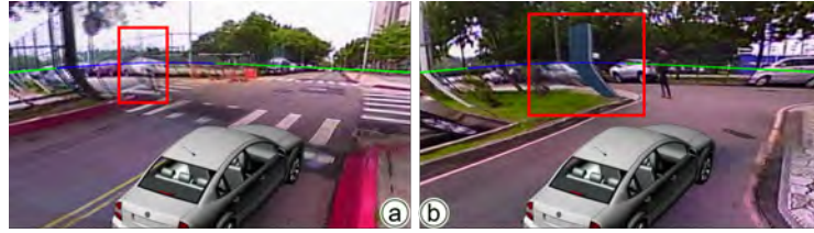
Fig. 17. Ghost effect and image distortion. The color line shows the seam between paraboloid model and columnar model, and the blue line shows the overlapping area. (a) Ghost effect. (b) Image distortion.
