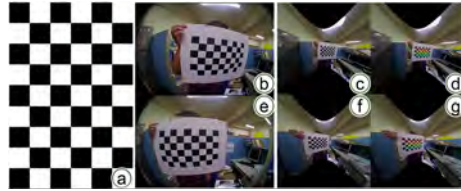
Fig. 6. (a) Chess board calibration pattern, (b)(e) the original fisheye images, (c)(f) undistorted images, and (d)(g) images in the calibration procedure.
