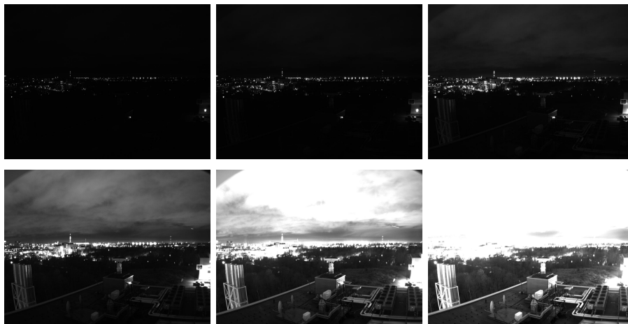
Fig. 4. Six subsequent images from an exposure time stack captured during a night. The exposure times are 72.9ms, 218.7ms, 656.1ms, 1.968s, 5.905s, and 11.810s.
