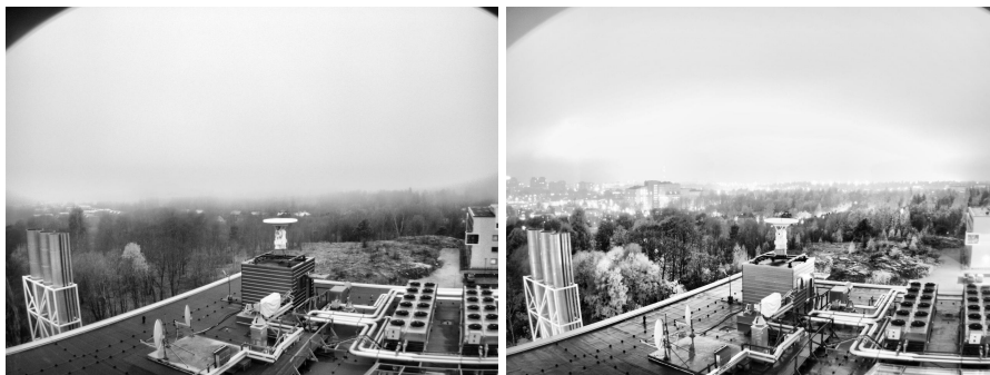
Fig. 1. Examples of cases where the light scattering equipment failed: (left,day) visibility measure 8180 meters and (right,night) 13 kilometers. The proper visibilities are less than 1000 meters and less than 5 km respectively. The clearly false measurements cause problems for example in aviation during day and especially at night.
