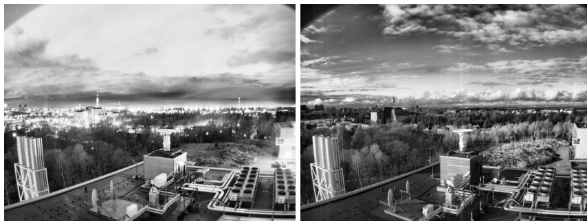
Fig. 5. HDR images obtained in a night and during a day. The images are tone mapped for viewing using contrast limited adaptive histogram equalization (CLAHE)[15].
