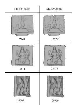
Fig. 10. Results for the proposed super resolution algorithm. Left column shows the 3D Objects of Low Resolution (LR) point cloud data. Right column shows the 3D Objects of Super Resolved (SR) point cloud data.
