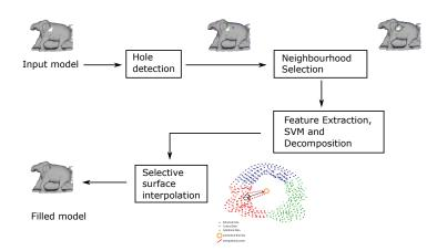
Fig. 6. Proposed hole filling algorithm.
