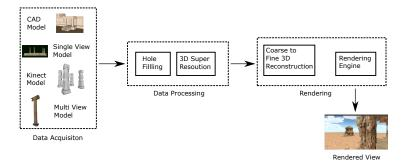
Fig. 3. Framework of coarse to fine 3D reconstruction and rendering to generate realistic walkthrough.
