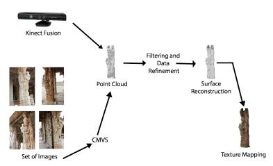
Fig. 4. Overview of the data acquisition and data refinement pipeline for detailed reconstruction.
