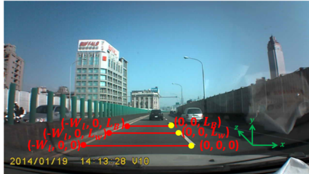
Fig. 5. The anchor points are used to estimate the camera pose.
