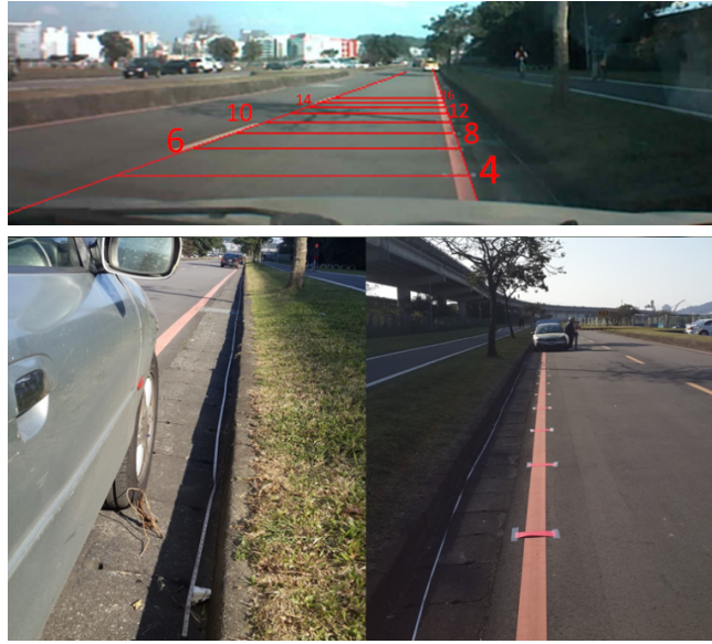
Fig. 7. It illustrates how the ground truth of distance estimation is obtained. The images are acquired from a vehicle video recorder. There are markers placed at 4, 6, 8, 10, 12, 14, 16, 18 m away along the side lane.
