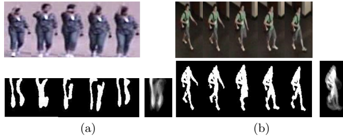
Fig. 4. GEI features extracted from sample sequences from the 2 datasets, (a) Lower body GEI from MCID dataset and (b) GEI from the SAIVT Soft-Bio dataset.
