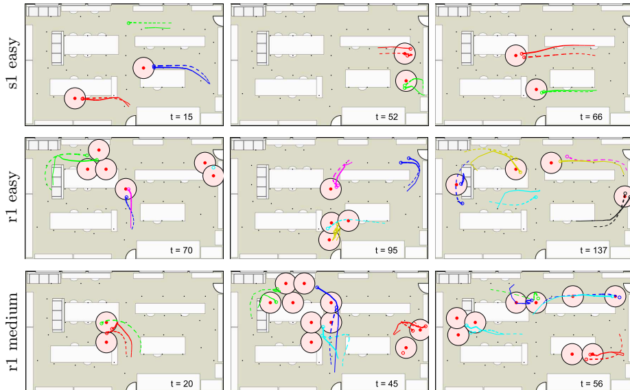
Fig. 3. Qualitative results on synthetic (top row) and real data (middle and bottom rows). 10 frames of both the recovered trajectories (solid) and the ground truth (dashed lines) are shown at three example time steps for each sequence. Note that despite the extreme amount of noise present in the observations (large circles), our method is able to successfully recover most of the targets’ trajectories.
