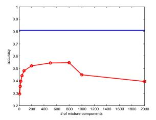
Fig. 4. Relationship between recognition accuracy and the number of mixture components for GMM-HMM (red line). The blue line is the final accuracy of CNN-HMM.
