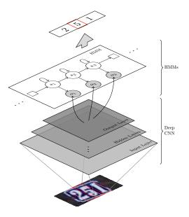
Fig. 1. Hybrid CNN-HMM Model. This image demonstrates the recognition process of our model. Input image is processed by sliding window to extract a sequence of frames. Each frame is normalised to the same scale and fed into the deep CNN which produce its posterior probability belonging to a category. This probability, after normalization, is used as the output probability of HMM. HMM is used to infer the most probable digits out of the frame sequence.
