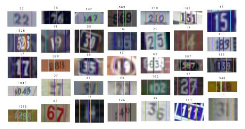
Fig. 6. Recognition results of hybrid CNN-HMM model. Segmentation line cuts generated by Viterbi algorithm are overlapped on the image. Two lines with the same color segment out a digit.
