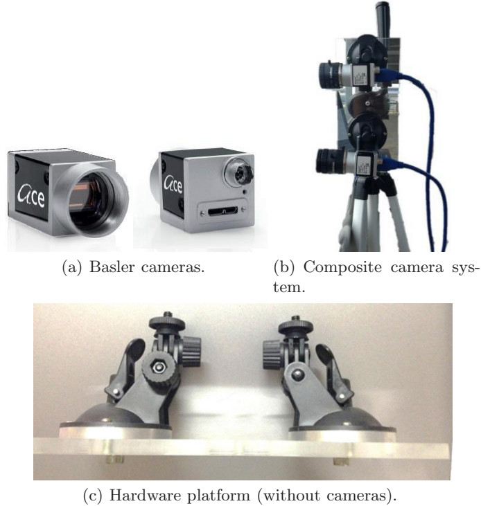
Fig. 6. Composite Camera built using USB 3.0 industrial cameras.
