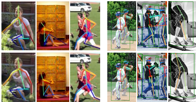
Figure 4: Examples of MDN-based improvements in human pose estimation through within-part voting (MPII dataset, Single person track , ResNet-152) on the left and cross-part voting (COCO dataset, Mask-RCNN-ResNet50-FPN) on the right. Top row: baseline performance, typical failure cases; bottom row: MDN-corrected body pose estimates.
