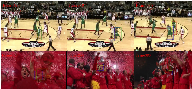
Figure 1: Tracking result comparison of our approach (green) with three state-of-the-art trackers (SiameFC is red, TCNN is blue, CCOT is yellow). As shown, in conditions such as occlusion, deformation, and cluttered background, the object appearance undergoes severe variations, DCTN outperforms the others thanks to the help of the motion cues.
