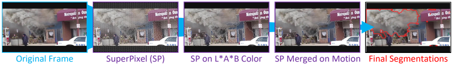
Figure 2: Steps in frame segmentation, each step uses agglomerative clustering to merge super-pixels into image segments; colour, motion and skeletal density are used respectively.
