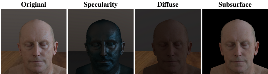
Figure 6: The non-specular component in case of a face scene can be further decomposed into only diffuse and subsurface scattering components.
