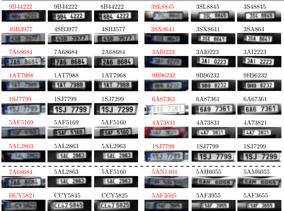
Figure 5: The first and the fourth columns show a sample of input images taken from the first frame of LR (60px) test sequences. The red strings denote the ground-truth. Other columns are super-resolution images created by the proposed CNN generator. The input of the generator was the corresponding LR image and the black strings shown above. The black strings were predicted from test sequences using LprNet-Avg(5) and they correspond to the MAP estimate and the second most probable hypothesis. The samples for which the MAP estimate of the string is correct are above the dash line. The samples below the line show errors. Note that the generated super-resolution images preserve structure of the LP inputs.
