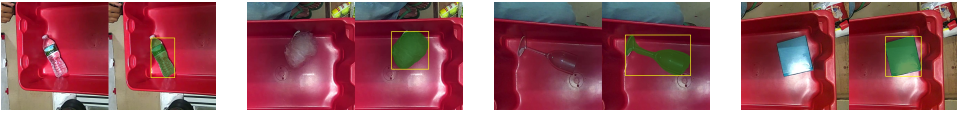
Figure 6: Figure illustrates few examples of binary mask generated using the proposed network. It can be observed that even for transparent objects the network can generate precise segmented region.
