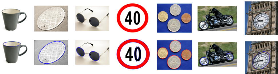
Figure 6: Test on real-life images: columns are tea cup, manhole cover, glasses, traffic sign, coin, motorcycle and big Ben images, and rows are the original inputs, the detected ellipses and circles overlaid on the input images. Note that all ellipses are rendered as blue while circle are rendered as red, and all images are scaled down to fit the page size.
