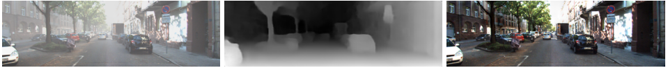
Figure 6: Simultaneous stereo matching and dehazing on the KITTI dataset [8]. (From left to right) Hazy left, estimated disparity, and dehazed image.
