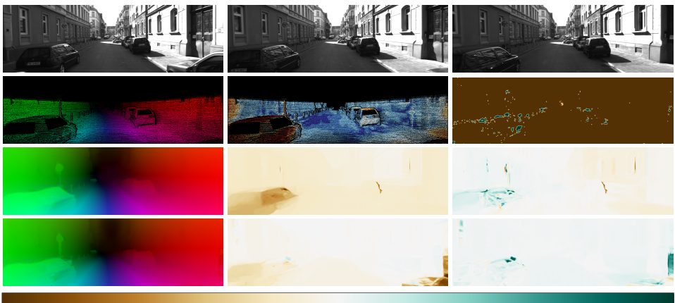
Figure 1: Exemplary result for a sequence of the KITTI 2012 [14] benchmark. First row: Input frames f^{t-1} , f^t and f^{t+1} . Second row: Ground truth forward flow, bad pixel visualization and computed order selection map o (first-order: turquoise, second-order: brown). Third row: Computed forward flow w^t , coefficients c_1^t and c_2^t (shifted and rescaled, zero maps to white). Fourth row: Computed backward flow w^{t-1} , coefficients c_1^{t-1} and c_2^{t-1} .
