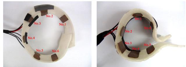
(a) Above-knee sensing front-end (b) Above-ankle sensing front-end
