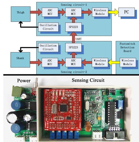
Fig. 4. The top half shows the structure of measurement system. The data flow is as follows, sensing circuit-2 detects the capacitance signals of shank and receives the data from footswitch detection board as well. It then transmits the data to sensing circuit-1. Sensing circuit-1 detects the signals of thigh and transmits all the data to the computer (PC). The bottom half shows the sensing circuit and power circuit.
