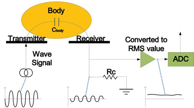
Fig. 1. Design concept of the prototype. The magnitude of the signal on the receiver electrode is influenced by the body movement. The signal was converted to RMS value before the ADC.
