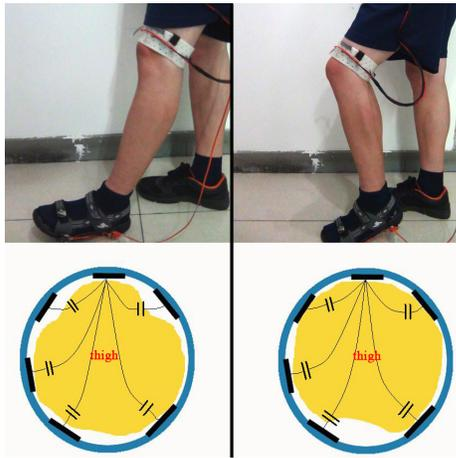
Fig. 3. The sensing principle of lower limb movement detection based on our prototype. The top half shows the flexion and extension of lower limb, and the bottom half shows the cross section of thigh accordingly. The shape change of thigh was reflected by the five channels of the capacitance signals. Note that the capacitive sensing system including two parts: above-knee module and above-ankle module. Here we only show the above-knee module for example.
