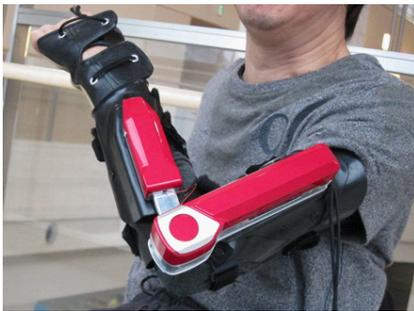
Fig. 1. Exoskeletal robot for the upper limb
