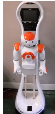
Figure 1: NAO and VGo Assembly.
