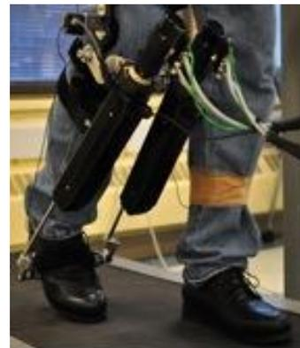
Fig. 1. Stroke participant undergoing Anklebot-assisted gait training on a treadmill. The Anklebot is providing plantar flexion push-off at the paretic ankle during mid-to-terminal stance, beginning with heel-off and peaking just prior to toe-off.
