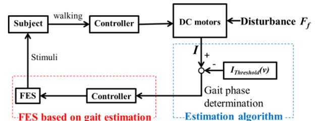
Figure 4. Block diagram of FES control based on gait phase estimation
