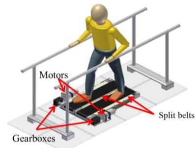
Figure 1. A split belt treadmill system for gait rehabilitation.
