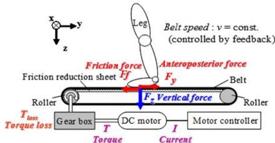
Figure 2. Mechanical model of walking on the treadmill belt.
