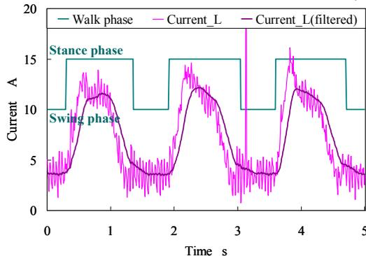
Figure 3. Walk phase estimation based on the motor current value.
