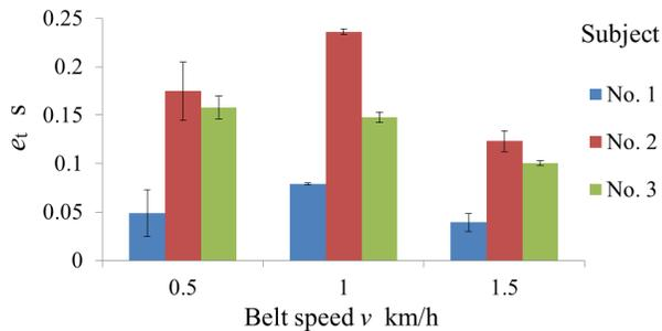
Figure 7. Timerror of stimulation control based on gait phase estimation and force plates for three subjects at three belt velocities.
