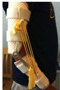
Figure 1. Mechanical rehabilitation brace for brachial plexus injuries.
