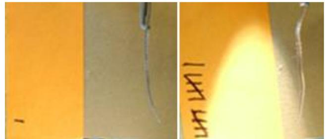
Figure 7. Cochlear implant with original stylet before ever being used (right) and after ten insertion trials and manual re-straightening (left). Note the significant shape change.
