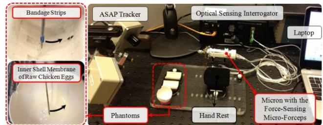
Figure 7. Setup for membrane peeling experiments on bandage phantom and inner shell membrane of raw chicken eggs.
