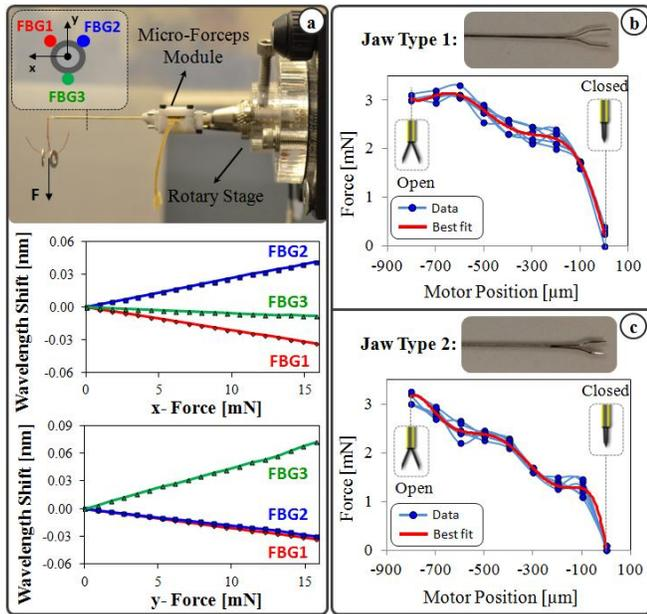
Figure 3. (a) Calibration results: Linear behavior is observed for all FBGs with tip loading in x-axis direction (upper) and in y-axis direction (lower). (b,c) Measured forces vs. the motor position while no external force is applied on the tool tip. Varying nonzero forces are observed due to inner actuation forces as the jaws are opened and closed. The force profile varies depending on the jaw type.
