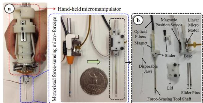
Figure 1. (a) Motorized force-sensing micro-forceps: earlier prototype [17] (left) vs. more compact new prototype (right). (b) Components of the new design: The tip can be easily replaced to accommodate different jaw types for different surgical tasks and prolonged use.
