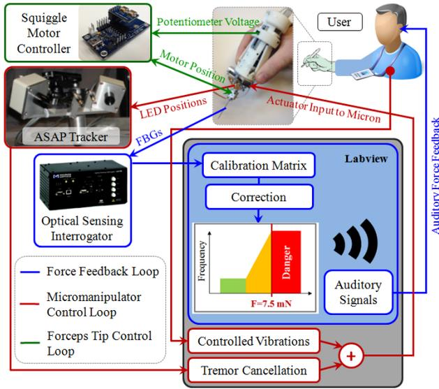
Figure 6. The control scheme of the integrated system. The existing tremor canceling control loop was extended to inject controlled vibrations for ease in membrane delamination. Opening and closing of the jaws are controlled via the potentiometer on the handpiece. Auditory force feedback is provided to the user to avoid excessive peeling forces.
