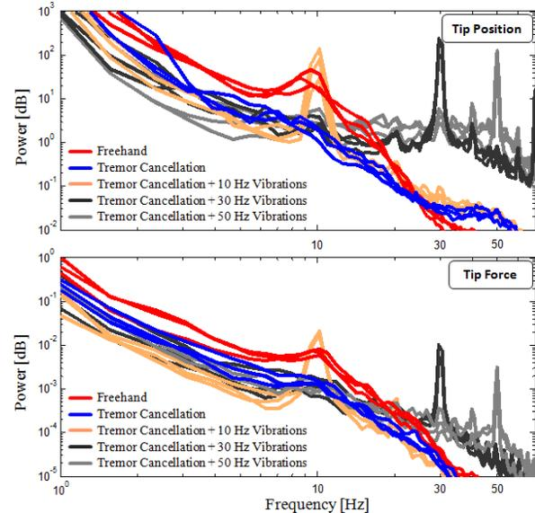
Figure 9. Power spectra of tip position and tip forces measured while peeling inner shell membrane of raw chicken eggs (3 arbitrary trials per set are shown). More deviation between trials as compared with bandage phantom, but the main traits were preserved: 45-90% and 5-85% reduction in 2-20 Hz band of tip position and force spectra respectively with tremor cancellation; visible peaks at 10, 30, and 50 Hz at both spectra.
