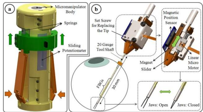
Figure 2. Design of force-sensing micro-forceps for handheld micromanipulators: (a) handle mechanism (b) motorized force-sensing tip with replaceable jaws. The tool can be inserted through a 20 Ga trocar into the eye. Squeezing the handle mechanism from the sides drives the motor and pushes the slide assembly forward, and thus closes the grasper jaws.
