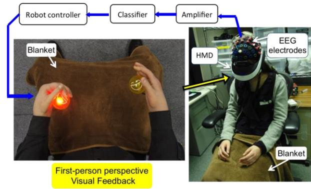
Fig. 1. EEG electrodes placed on subject's sensorimotor cortex recorded brain activities during a motor imagery task. Subjects watched first-person images of robot's through a head mounted display. A lighting ball in front of robot's hands gave motor imagery cue and subjects held images of a grasp for their own corresponding hand. Classifier detected two classes of results (right or left) and sent a motion command to robot's hand.
