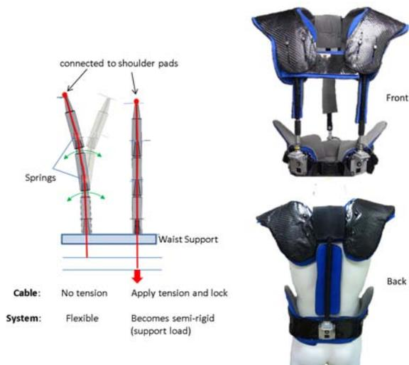
Fig. 1. Cone-shaped joints allow two segments to share the maximum area of contact when they are pulled together by a cable routed from the top segment to the bottom. Springs are interposed between two mating segments to ensure separation when the cable is not tensioned (left). Prototype of the Second Spine (right) [18].
