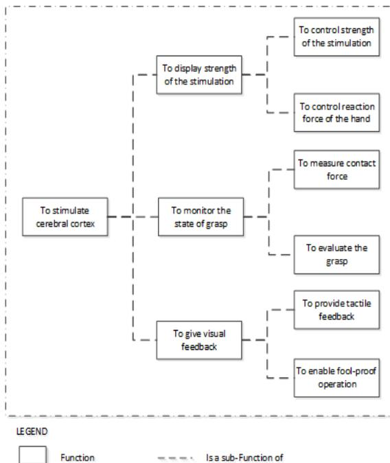
Figure 5. Function of Hand Rehabilitation Device System (HRDS)
