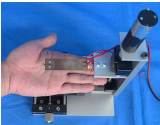
Figure 12. The experimental setup to evaluate the tactile area of the palm.
