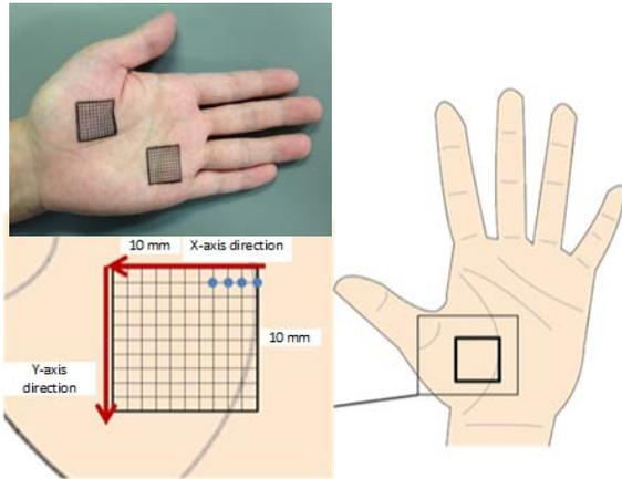
Figure 10. The tactile area subjected on the palm in the measurement.
