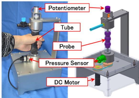
Figure 4. The conceptual design of HRDS
