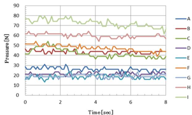
Figure 9. Grasping pressure variation for 9 healthy subjects while gripping the rotational shaft which stimulates the palm at a rate of stimulation of 50 RPM
