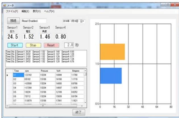
Figure 7. Interface of data logger system for assessment tools
