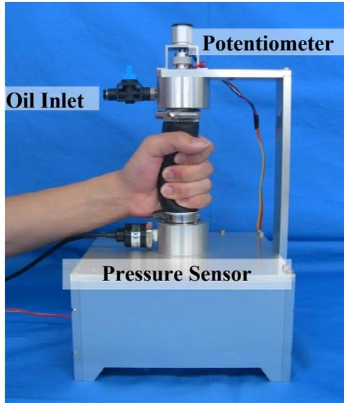
Figure 6. Rehabilitation device to stimulate the sensory function.
