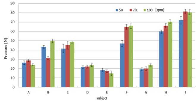
Figure 8. Grasping pressure for 9 healthy subjects while gripping the rotational shaft which stimulate the palm at stimulation rates of 50,70 and 100 RPM
