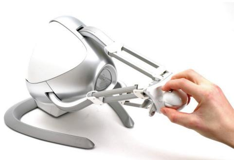
Fig. 1. Novint Falcon haptic manipulator.
