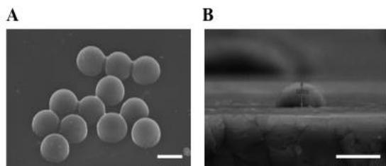
Fig. 3. SEM images of submerged PS microbeads on PDMS surfaces of (A) 3.0 kX magnifications and (B) 5.0 kX magnifications at 15.0 kV (Scale bars = 5  $\mu\text{m}$ ).
