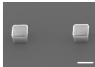
Fig. 1. SEM Photographs of 30 µm SU-8 microcubes on silicon wafer at 15.0 kV and 600 X magnifications after microfabrication (Scale bars = 30 µm).
