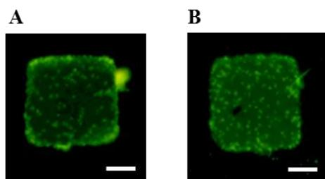
Fig. 2. Fluorescent microscopic images of green fluorescent staining *S. marcescens*-attached SU-8 microcubes. (A) BSA-untreated bottom side of SU-8 microcube and (B) BSA-treated bottom side of SU-8 microcube (Scale bars = 10  $\mu\text{m}$ ).
