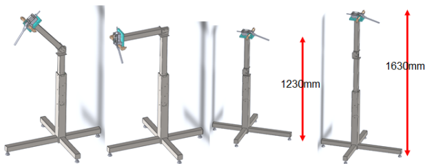
Fig. 5. Solidworks drawing of the total mechanical design: supporting holder of RFLS can be adjusted in height and direction.
