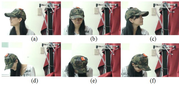
Fig. 11. Snapshots of the experiment: The motion sensor that measures the head orientation is worn on top of the head. User rotates his/her head to control the laparoscope. (The laparoscope can be moved with 8 difference orientations.)
