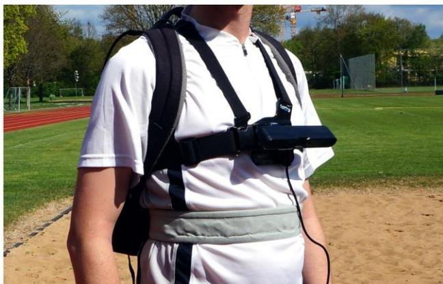
Figure 2. Test setup of the course detection, worn by a test person, with the Asus camera, attached with a modified GoPro belt, the belt based feedback system and a laptop in a rucksack as processing unit.
