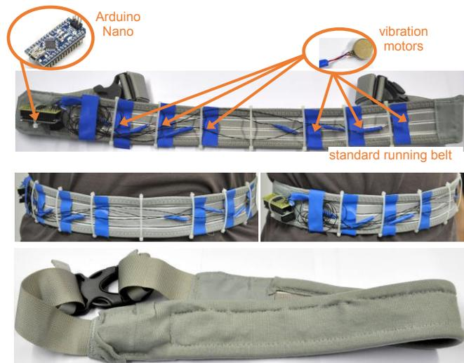
Figure 4. First prototype of the belt feedback system, based on a standard running belt, six vibration motors and an Arduino Nano. The three pictures at the top show the motors only fixed by tape, in the subsequent version (image at the bottom) they are sewed into inlets by flexible fabric.
