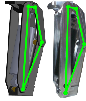
Fig. 2. CAD drawing (left) of the knee prosthesis and the real mechanism (right). The green lines show the four-bar linkage mechanism.
