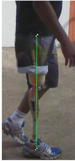
Fig. 4. Amputee subject using the prototype illustrating the load line (green line) position with respect to the ICR (intersection between the red dash lines).
