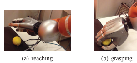
Fig. 8. The reaching and grasping configurations performed by the robotic arm-hand system.
