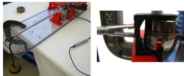
Figure 3. Instrument in test bed for calibrating forces in the  $x$  and  $y$  axes (left) and for calibrating the grasping force (right).
