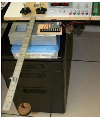
Figure 1. Experimental jig with stainless steel bar in cantilever.
