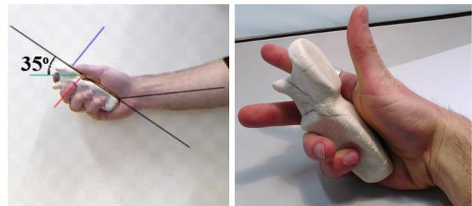
Fig. 11. Left: Grabbing axes analysis. Right: Fingers' angle
