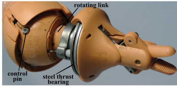
Fig. 6. Grasper assembled with the steel thrust bearing
