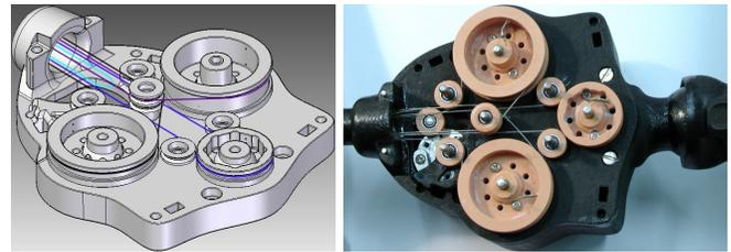
Fig. 8. Gearbox assembly with wires setup
