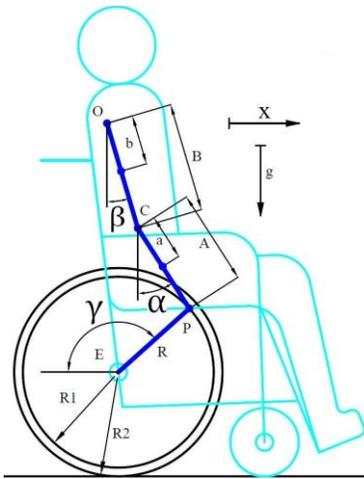
Figure 1 – Schematic representation of wheelchair/user model.
