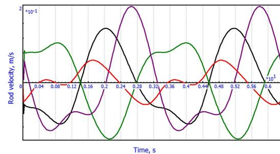
Fig. 9: Velocity of the exoskeleton cylinder rods for the left leg
