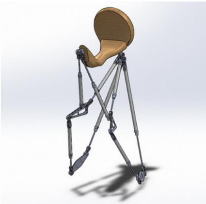
Fig. 4: Lower limb exoskeleton 3D model
