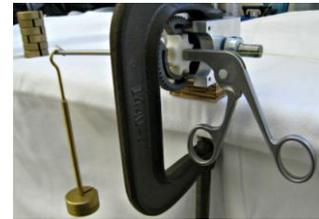
Figure 6. Bending calibration apparatus.
